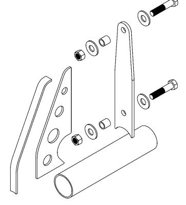
11...Bolt the mid plate to the mounts using the 3/8"bolts, washers and stover nuts.
